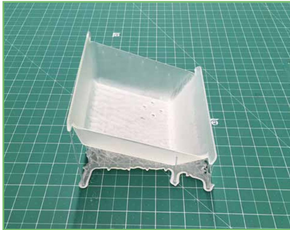
Model out of the SLA printer, very rough surfaces.
