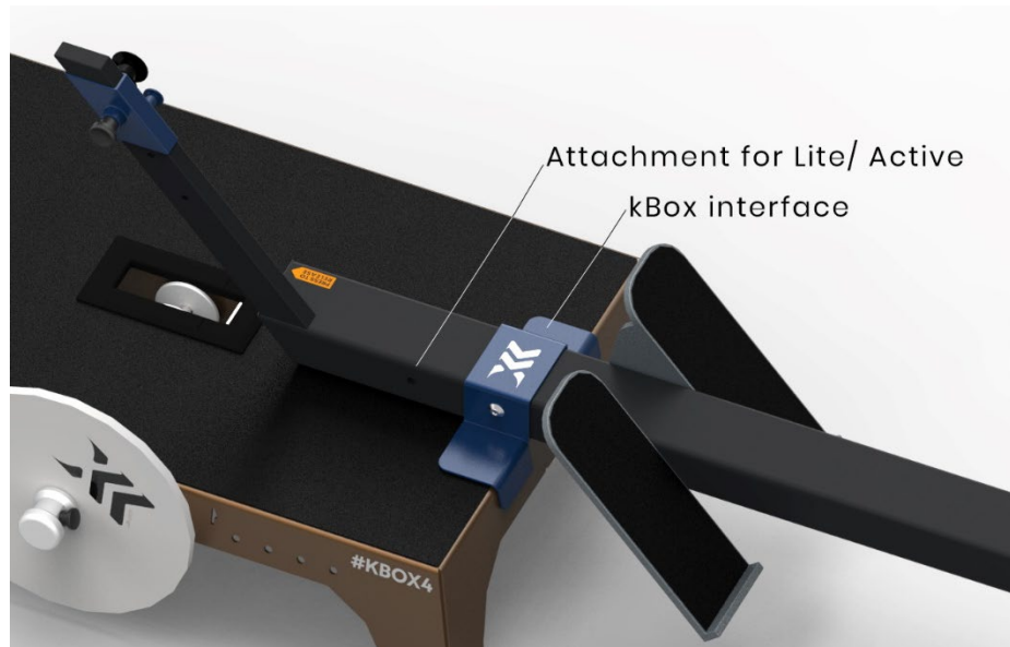
Figure 6.17. Interface on kBox provided support and stability in addition to acting as a guidance as to how far the add-on should overlap with the kBox.
