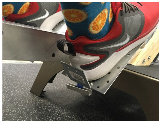
Figure 6.6. Prototype heel support for the foot plates.
